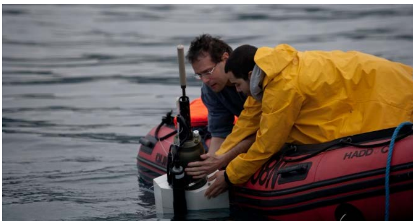
© Antoine Poteau, Observatoire Océanologique de Villefranche (CNRS/UPMC) Deployments of a bio-Argo Provor in Ligurian sea
