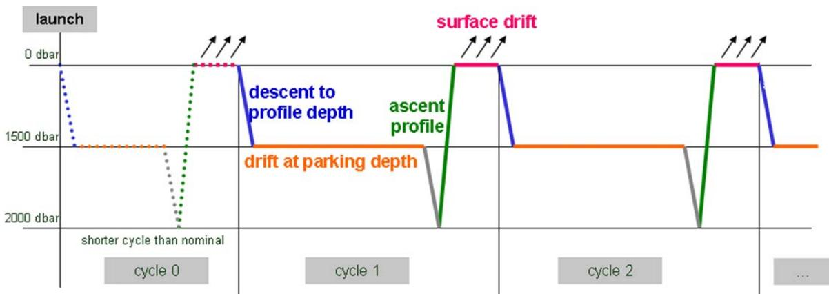
**A typical Argo float performs continuously measurement cycle during 3 years or more in the ocean.**
