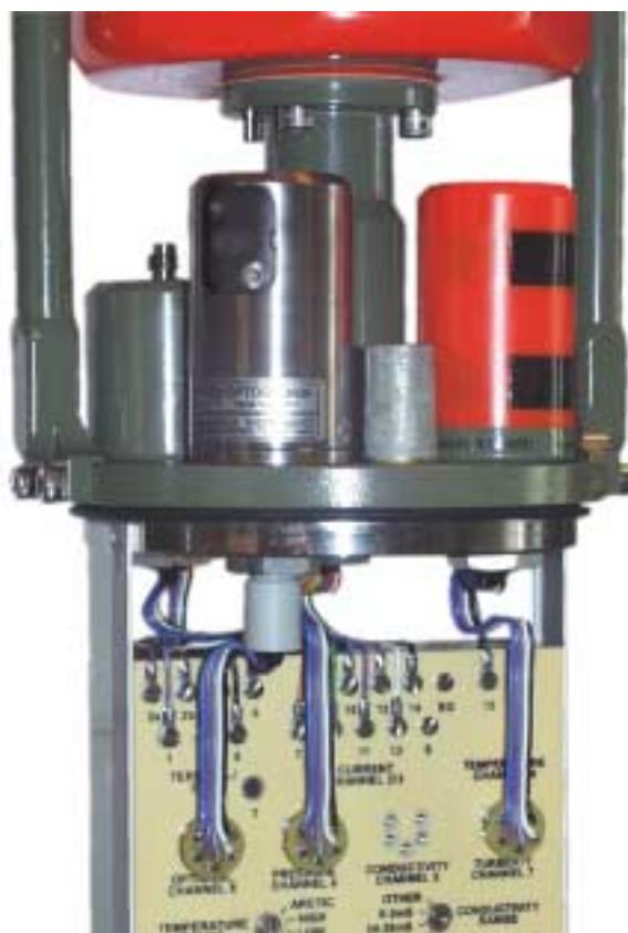
Fig. 6.04 Sensor connected to Electronic Board
