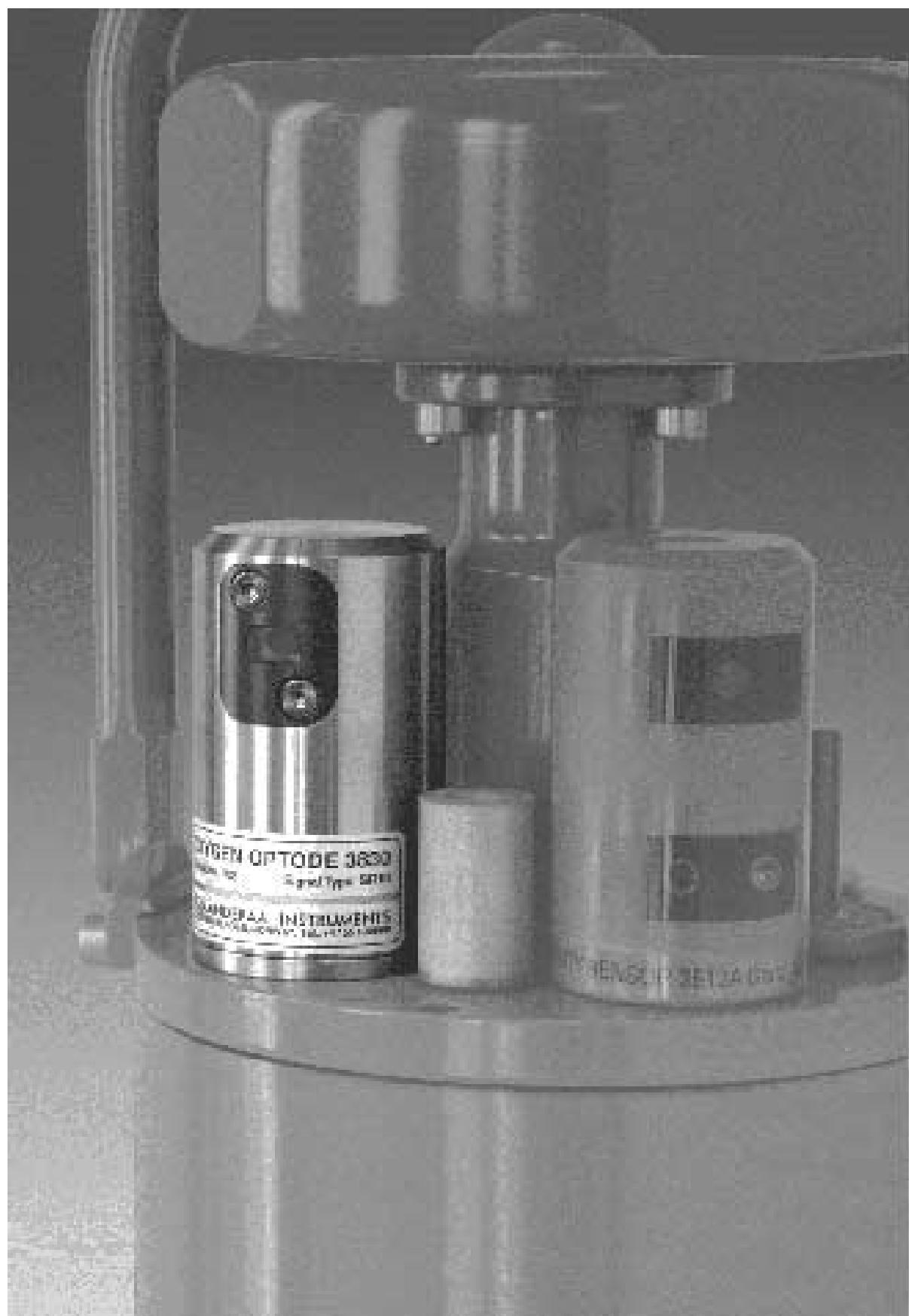
*Fig. 0.01 Oxygen Optode 3830 mounted on an RCM 9 MkII*
