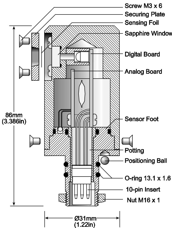
Fig. 6.02 Drawing of Sensor
