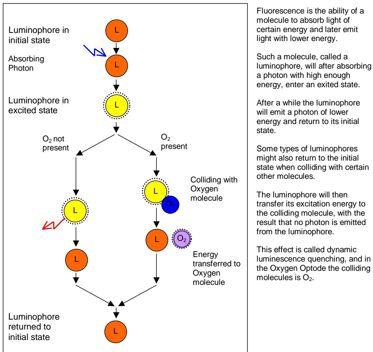
Fig. 2.01 Dynamic Luminescence Quenching
