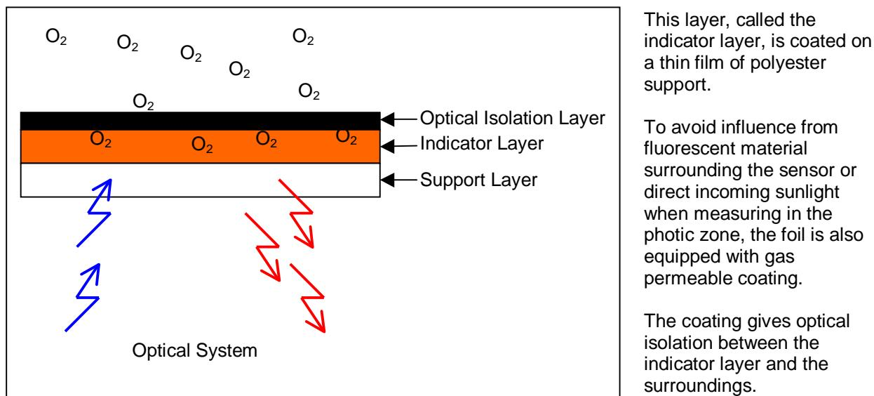
Fig. 2.02 Sensing Foil
