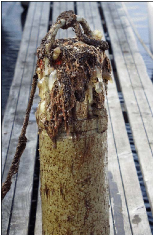
Figure 6-1 Example of fouling on an RCM 9 with an Oxygen Optode 3830 (Optode version with SR-10 output) mounted to it: The Optode was still giving correct readings.
