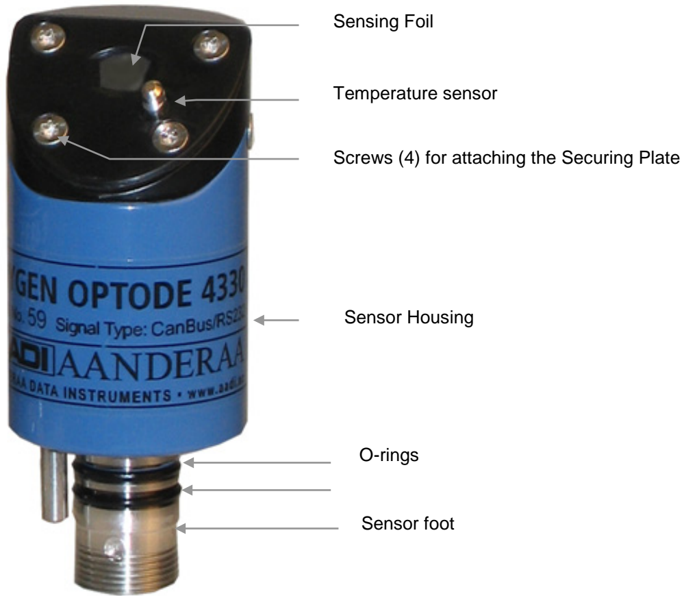
Figure 1-1 Illustration of the Oxygen Optode 4330.
