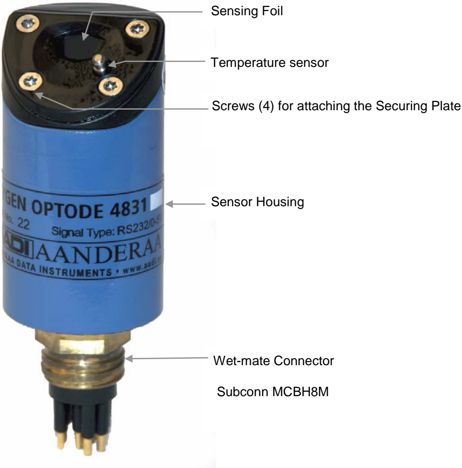
Figure 1-2 Illustration of the Oxygen Optode 4831
