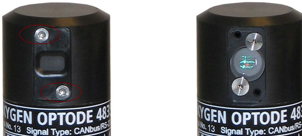
Figure 5-4 Removing the securing plate and change the sensing foil.
