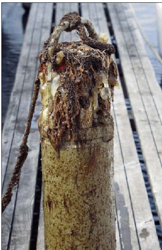
Figure 5-1 Example of fouling on an RCM 9 Mk II with an Oxygen Optode 3830 (optode version with SR-10 output) mounted to it: The optode was still giving correct readings.
