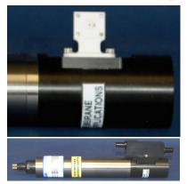
processes, especially when water temperature is changing rapidly, is a key accomplishment of the design. Not only does the SBE 43 sensor measure temperature in the right place: the temperature equilibration time of the entire sensor head has been reduced to a few seconds, so it tracks changing water temperature much more faithfully.
