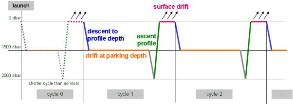
A typical Argo float performs continuously measurement cycle during 3 years or more in the ocean. A more detailed cycle description is available in reference table 15, chapter 3.15.
